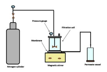
Fig. 1. Schematic of dead end system.
