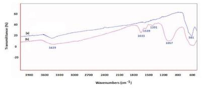
Fig. 2. FTIR spectra of unmodified (a) and CC modified Fe<sub>3</sub>O<sub>4</sub> particles (b).
