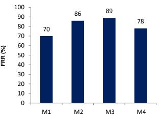
Fig. 5. Water flux recovery of the Fe<sub>3</sub>O<sub>4</sub>/OCMCS nanoparticles blended PES membranes after activated sludge suspension fouling. (Average of three replicates was reported).
