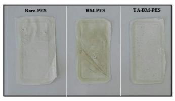
Fig. 13. The photo of nanocomposite membrane after licorice fouling.
