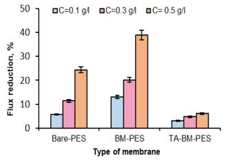
Fig. 12. The results of flux reduction ratios of NF membranes at various feed composition.
