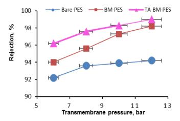
Fig. 6. Influence of operational pressure on rejection of nanofiltration membranes (C=0.3 g/L, time=30 min, V=1 cm/s).
