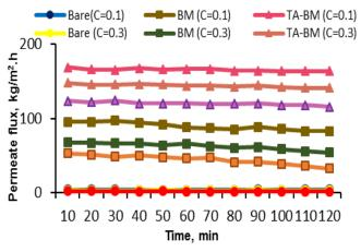
Fig. 11. The permeated flux profile against filtration time of nanofiltration membranes (P=6 bar, time=120 min, V=1 cm/s).
