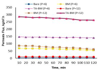
Fig. 4. The permeated flux profile versus filtration time of nanofiltration membranes (C=0.3 g/l, time=120 min, V=1 cm/s).
