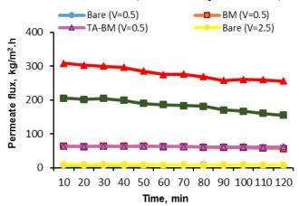
Fig. 8. The permeated flux profile against filtration time of nanofiltration membranes (C=0.3 g/l, time=120 min, P=6 bar).
