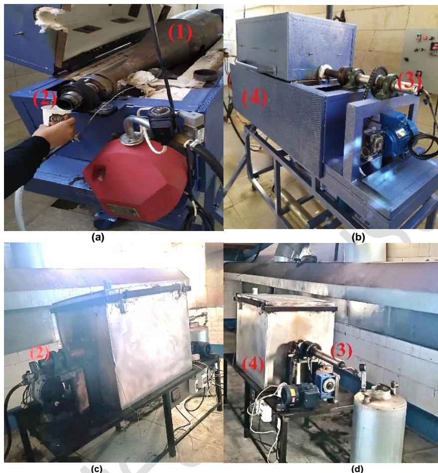
Fig. 1. Rotary furnace system for wool activation: (a-b) 3-liter unit and (c-d) 7-liter pilot-scale unit. Rotating tank, discharge outlet, steam inlet and the double-wall insulated heater housing are identified with numbers (1) - (4) respectively.
