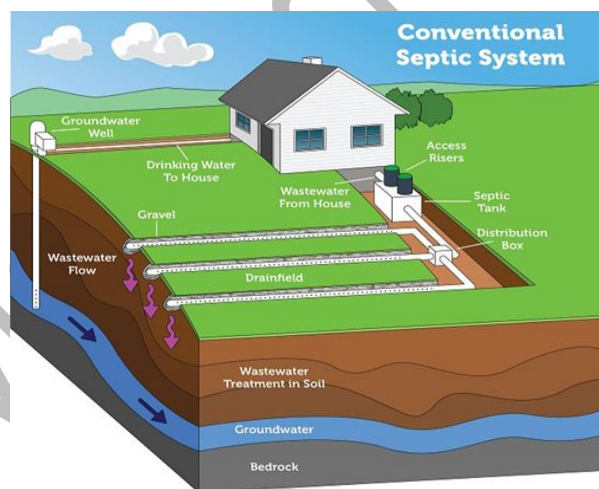
Fig. 3. The conventional septic system.
