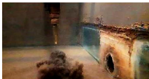
Fig. 6. Submerged jet flow to improve flushing efficiency (Madadi et al. 2018).
