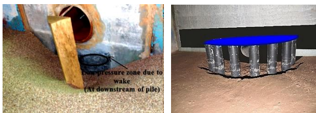
Fig. 3. Installation of piles behind the low-level outlet to improve the flushing efficiency; single pile (left), semi-confined pile group structure (right) (Madadi et al. 2016; Beyvazpour et al. 2021).
