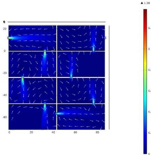
Fig. 1. Velocity distribution in existing CW.
