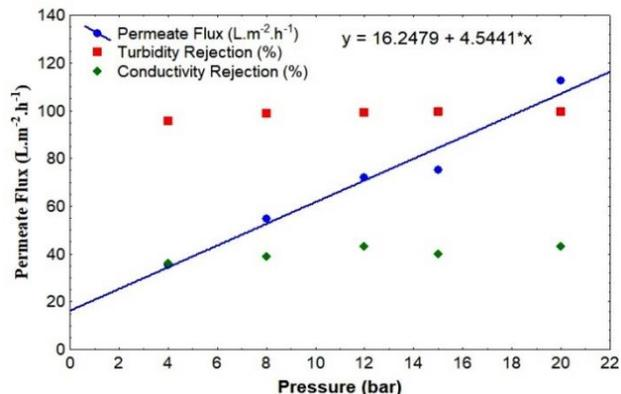
Fig. 16. Permeate flux, salt and turbidity rejection of the oxidized membrane in 10,000 ppm.h treating surface water from St Nicolas Dam river (France).
