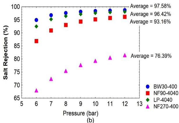
Fig. 6. (a) Salt rejection of the aged and oxidized membranes; (b) Salt rejection of references membranes simulated on ROSA software.
