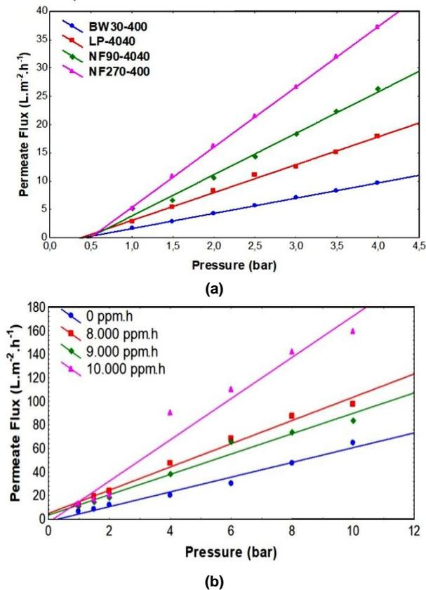
Fig. 4. Permeate flux at different pressures (a) of the aged RO and oxidized membranes and (b) Simulation of permeate flux of membranes references on ROSA software.
