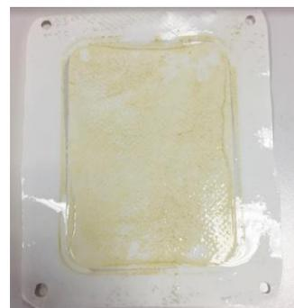
Fig. 17. Picture of the oxidized membrane in 10,000 ppm.h of chlorine after treating surface water.
