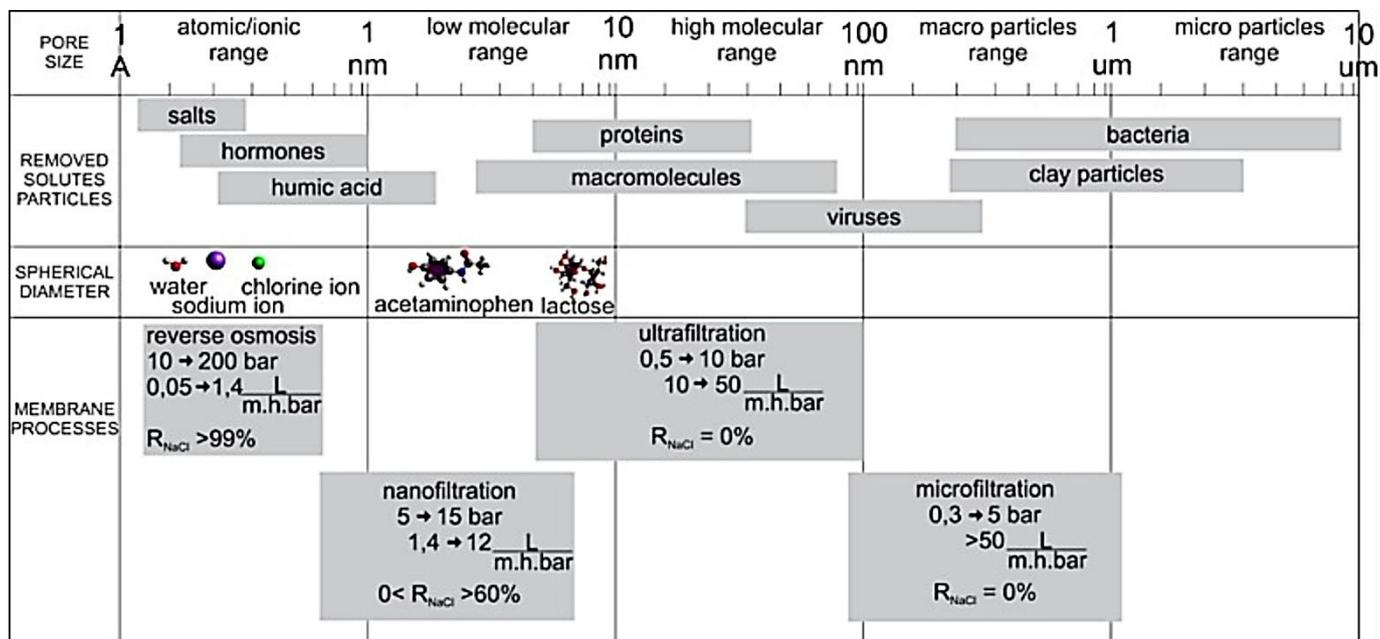
Fig. 1. Characteristics of pressure driven membrane separation process and some substances usually separated by each process. Adapted from Warsinger et al. (2018).
