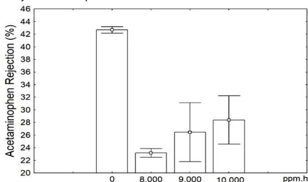
Fig. 9. Acetaminophen rejection of the aged and oxidized membranes.
