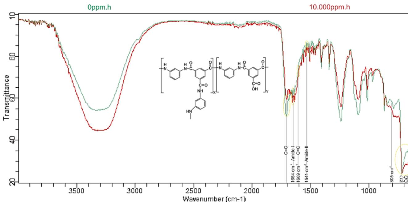
Fig. 13. FTIR of the aged RO membrane (green line) and oxidized membrane (red line).
