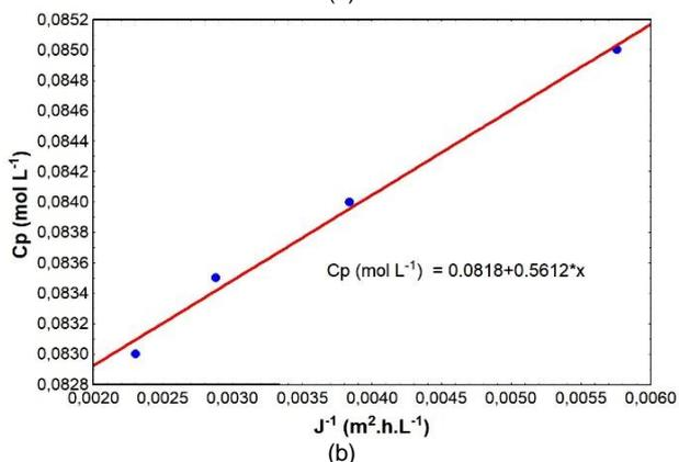
Fig. 7. Salt concentration in permeate versus inversed flux ( $J^{-1}$ ), for prediction of diffusive and convective mass transfer across the aged (a) and oxidized in 10,000 ppm.h (b) membranes.
