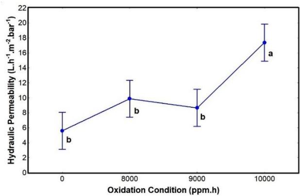
Fig. 5. Average hydraulic permeability of the aged RO membrane and oxidized membranes.
