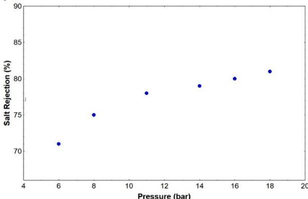
Fig. 15. Salt rejection of the oxidized RO membrane in 10,000 ppm.h when treating brackish water.
