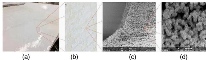
**Fig. 2.** (a) and (b) pictures of the membrane during the autopsy procedure of the aged membrane, (c) and (d) scanning electronic microscopy (SEM) of the aged membrane at 20 μm and 1 μm, respectively.
