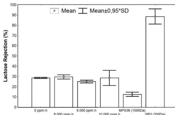
Fig. 8. Lactose rejection of the aged, oxidized and references NF membranes.
