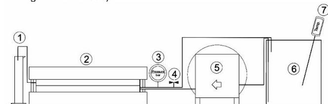
**Fig. 3.** Schematic of the bench-scale membrane test cell, (1) graduated cylinder, (2) test cell, (3) pressure gauge, (4) recirculation valve, (5) pump, (6) feed solution storage beaker, (7) thermometer.
