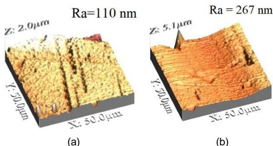
Fig. 12. SEM image and AFM analysis of the (A) aged RO membrane and the (B) membrane oxidized in 10,000 ppm.h of Cl<sub>2</sub>.
