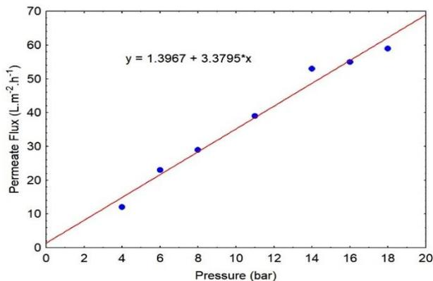
Fig. 14. Permeate flux of the oxidized RO membrane in 10,000 ppm.h when treating brackish water.
