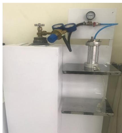
Fig. 1. The dead-end setup schematic shape.
