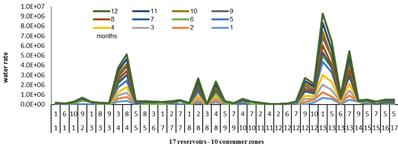
**Fig. 4.** Amount of water transfer from reservoirs to consumer zones in all of 12 months (m<sup>3</sup>).
