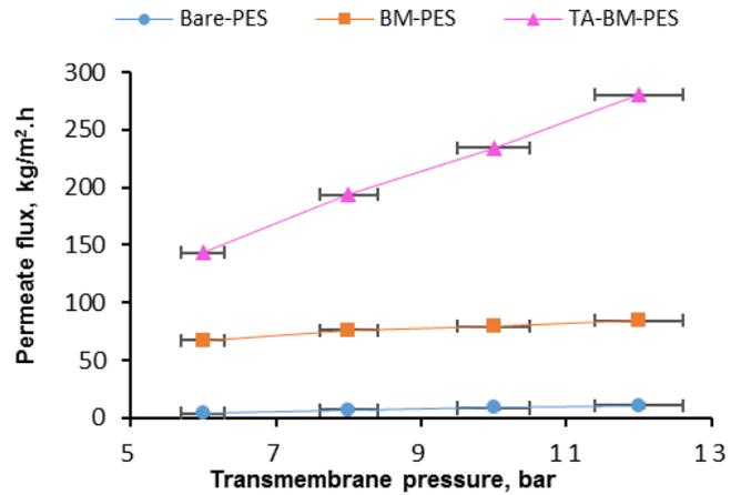
Fig. 3. Influence of operational pressure on permeation flux of NF membranes (C=0.3 g/L, time=30 min, V=1 cm/s, pH = 5.3).
