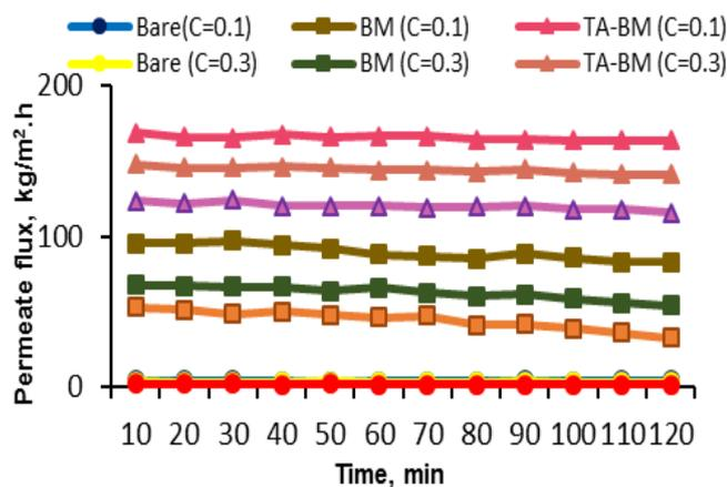
Fig. 11. The permeated flux profile against filtration time of nanofiltration membranes (P=6 bar, time=120 min, V=1 cm/s).
