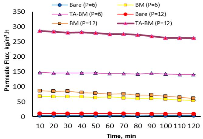
Fig. 4. The permeated flux profile versus filtration time of nanofiltration membranes (C=0.3 g/l, time=120 min, V=1 cm/s).
