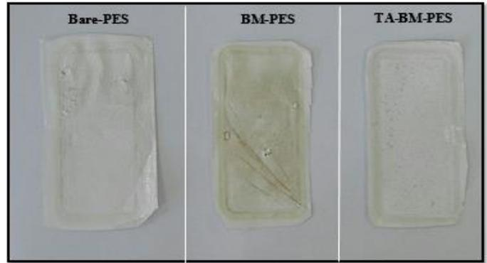
Fig. 13. The photo of nanocomposite membrane after licorice fouling.
