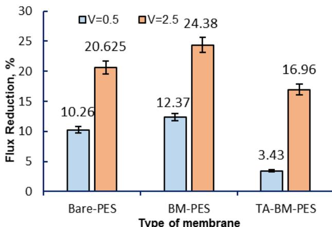
Fig. 9. The results of flux reduction ratios of NF membranes at diverse cross-flow velocity.
