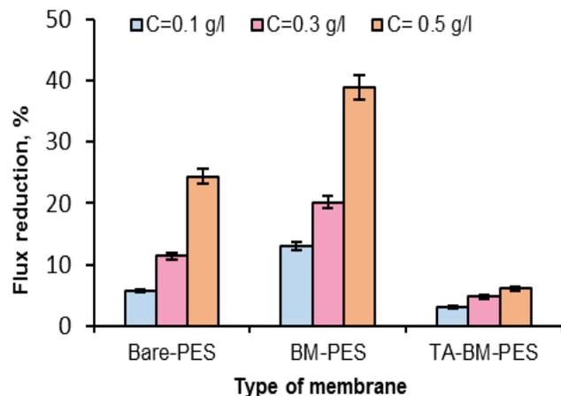
Fig. 12. The results of flux reduction ratios of NF membranes at various feed composition.
