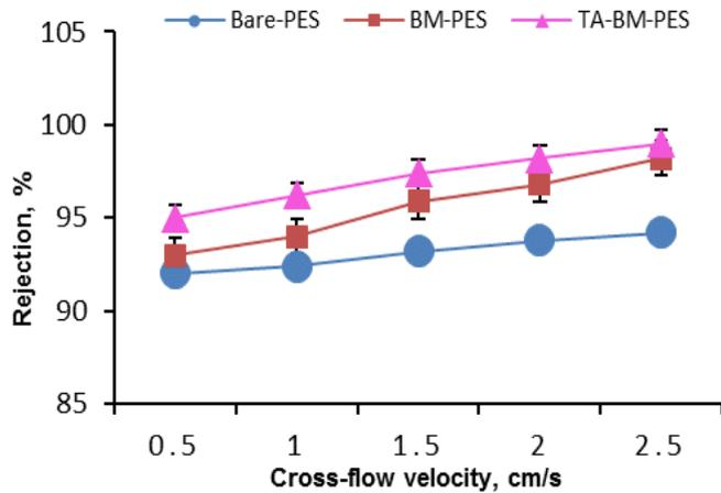
Fig. 10. Influence of cross-flow velocity on rejection of nanofiltration membranes (P=6 bar, C=0.3 g/l, time=30 min, PH = 5.3).
