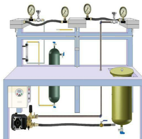
Fig. 1. The schematic of cross-flow filtration system.
