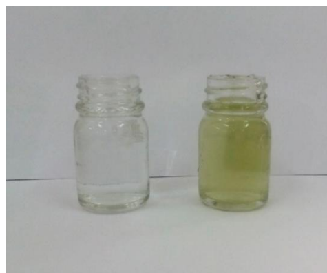
Fig. 5. Comparison of the wastewater appearance before (right) and after membrane treatment (left).
