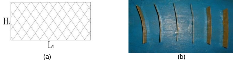
Fig. 3. (a) Characteristics submerge vane ; (b) Six types of curvature submerged vanes.
