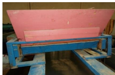
Fig. 2. (a) Gradation curve of the injected sediments to the vortex settling basin with d50=0.22mm; (b) Sediment injection machine.
