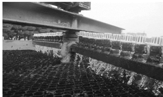
Fig. 4. Rotary sprinkle system on the pilot head.
