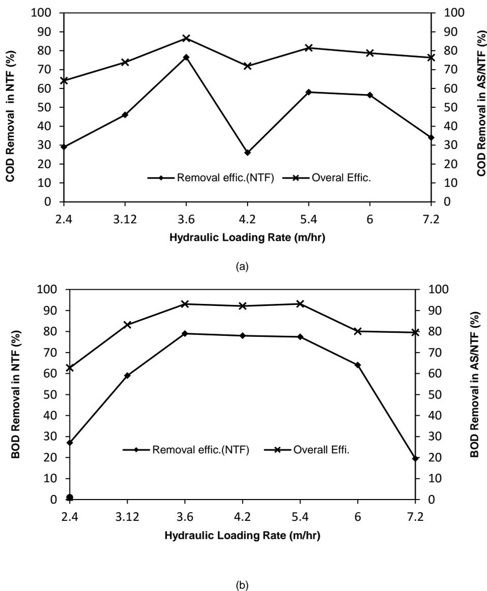
Fig. 5. Removal efficiency of organic compounds in NTF and AS/NTF Versus HLR, (a) COD and (b) BOD<sub>5</sub>.
