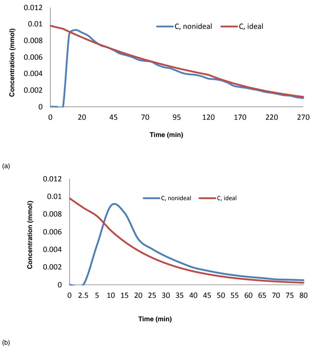
Fig. 2. Mathematical and empirical curves of tracer concentration time distribution for (a)  $V_{up}=0.5$  m/h and  $Q_g=14.87$  l/d, (b)  $V_{up}=3.0$  m/h and  $Q_g=7.96$  l/d.
