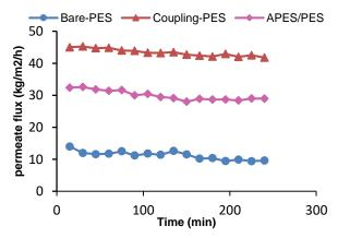
Fig. 5. The long term performance of the membranes at optimum condition (p=6 bar, v=1.5 cm/s, PH = 5.3).
