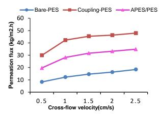
**Fig3.** Impacts of cross-flow velocity on permeation flux of membranes (p=6 bar, PH = 5.3).
