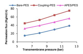
Fig.1. Impact of transmembrane pressure on permeation flux of membranes (v=1.5 cm/s, PH = 5.3).
