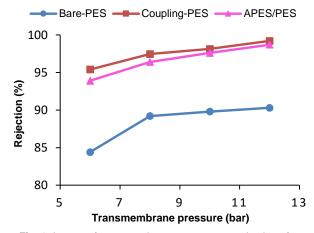
Fig. 2. Impact of transmembrane pressure on rejection of membranes (v=1.5 cm/s, PH = 5.3).
